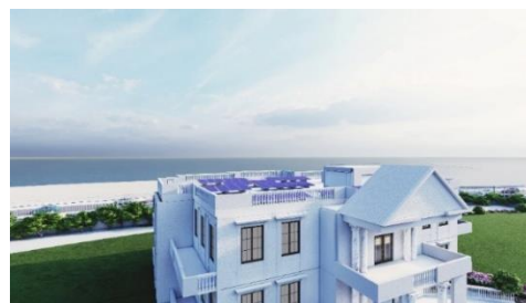
Figure 15. shows the solar panels added to the roof in the direction of south and southeast direction to enhance the energy efficiency of the building. Source: By authors using Revit software.
