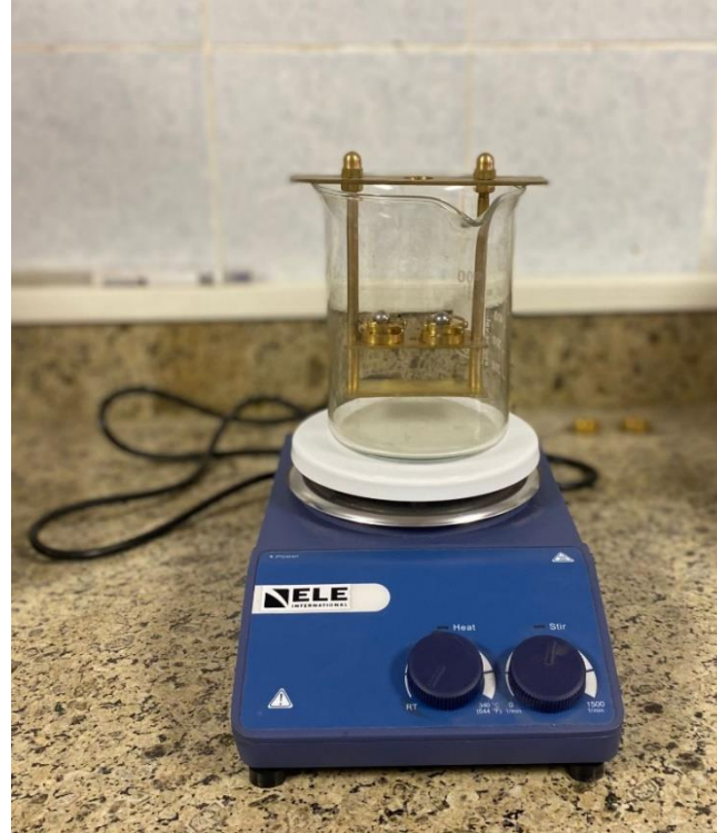
Ring and ball test
